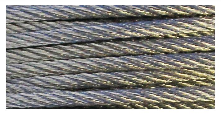
In hot dip galvanized cable, each uncoated steel wire is immersed in a molten zinc bath. Prior to dipping, the wires are put through a rigorous 7-step caustic cleaning process and then dipped into the molten zinc at a temperature of around 860°F/460°C. As it's withdrawn from the molten bath, the material cools and forms a coating of zinc on the steel. The wires are then formed into strands and then the strands are helically formed into the finished cable or wire rope configuration.
