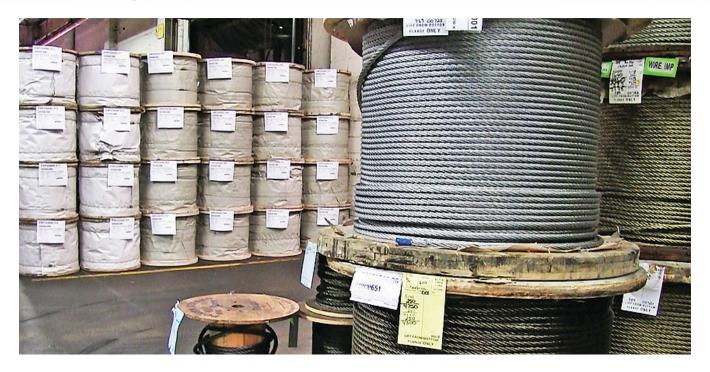
The term "galvanized" only tells the end-user that some type of corrosion-resistant coating has been applied to the steel material. However, suppliers don't always specify whether the cable they're selling is an electro galvanized or a hot dip galvanized product.
