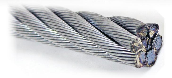
For extreme environments where exposure to moisture, salt water, or corrosive or caustic chemicals is possible, the correct type of stainless steel cable is the preferred choice. For most applications, a galvanized zinc coating will offer some form of corrosion resistance and still provide the strength and flexibility characteristics desired by the end-user.
