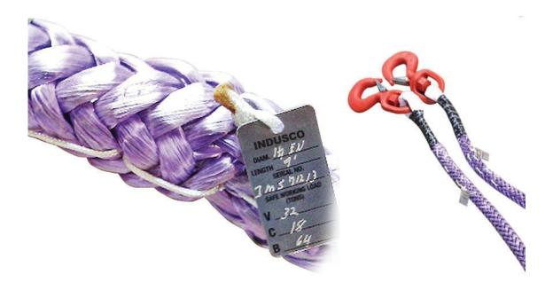
Synthetic rope sling identification shall be done by the sling manufacturer, but should be maintained by the user so as to be legible during the life of the sling.
