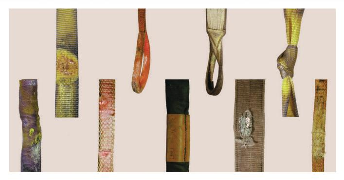
Careful consideration must be given to the application when determining whether or not to use a synthetic lifting sling. They are more susceptible to damage from environmental factors like extreme temperatures, prolonged UV exposure, and chemically active environments. They're also not as durable as steel wire rope slings or alloy chain slings when it comes to abrasion and cut resistance.
