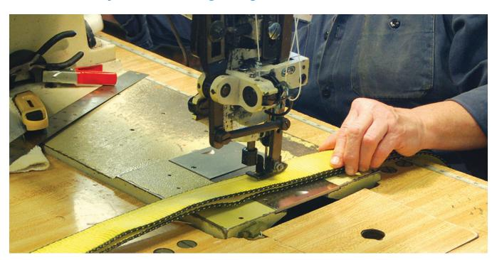
If you're lifting highly finished parts or delicate materials, then a synthetic lifting sling can provide the flexibility, strength, and support you need to support a specialized load. Synthetic slings can be made from polyester, nylon, or high-performance materials and are lightweight, easy to rig, and extremely flexible.
