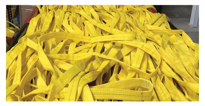
Web slings are flat belt straps made of webbing material and most commonly feature fittings, or flat or twisted eyes, on each end. Web slings are the most versatile and widely-used multi-purpose sling. They're strong, easy to rig, and inexpensive. Compared to chain, they're more flexible and lighter and can be used to help reduce scratching and denting to loads. They can also be fabricated with wide load-bearing surfaces up to 48" to provide significant surface contact for heavy and large loads.
