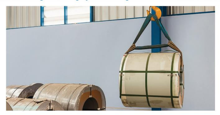
Because they're so flexible, they can mold to the shape of delicate and irregularly-shaped loads, or be used in a choker hitch to securely grip loads of round bar stock or tubes. The soft materials they're made from are strong enough to lift heavy loads, but will protect expensive and delicate loads from scratches and crushing.
