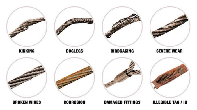
This being said, inspection of wire rope most often uncovers broken wires, corrosion, and distortion of the rope's original structure (kinking, crushing, or birdcaging). Any type of distortion that doesn't straighten itself out when the rope or sling is put under load is cause for removal from service.
