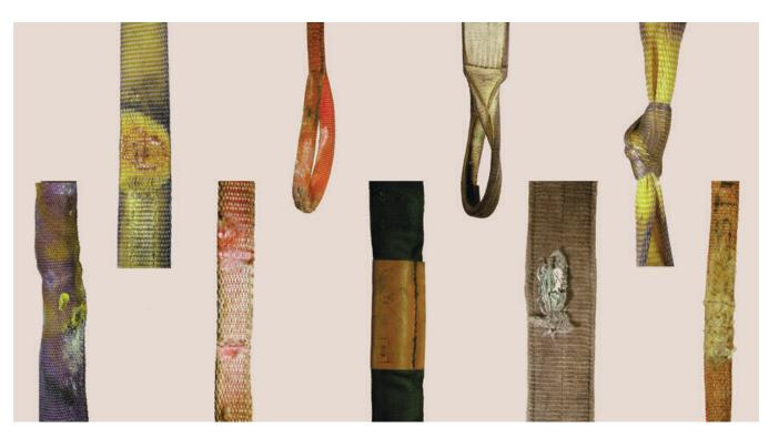
Synthetic web slings and roundslings—made from nylon or polyester—are more susceptible to damage from environmental factors like extreme temperatures, prolonged UV exposure, and chemically active environments. They're also not as durable as steel wire rope slings or alloy chain slings when it comes to abrasion and cut resistance.
